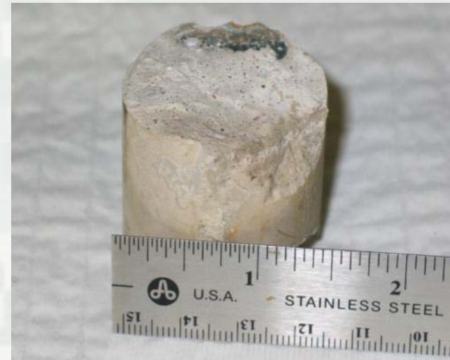
Soil solidified with alkali-activated mixture using slag
