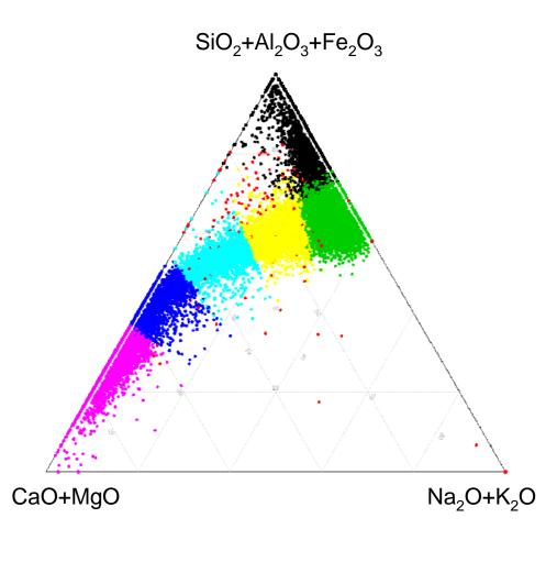
Table 1 Classification of Glassy Phase based on Cluster Analysis of Coal Creek Fly Ash
