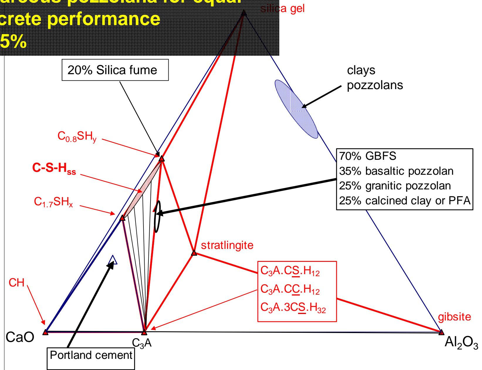
Max clinker replacement by non-calcareous pozzolans for equal concrete performance
