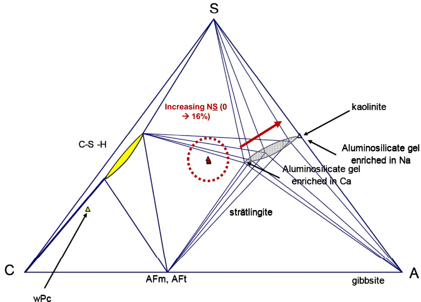
40% clinker, MK/(MK+ls) ratio = 0.96, sodium sulfate content = 0, 4, 10, 16%
