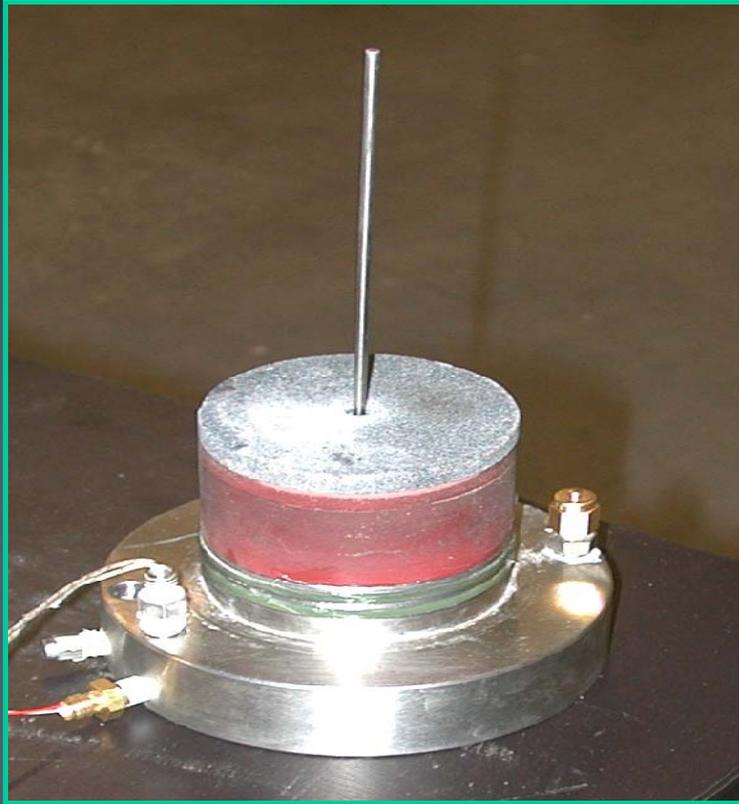
*Base platform with axial heating source*
