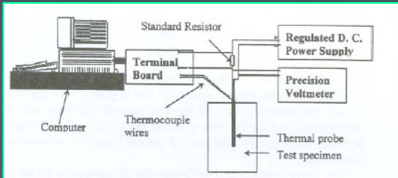
*Schematic of electrical circuit and data acquisition system at the University of Alberta*
