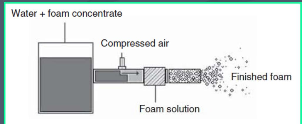
*Schematic of a foam generator*
