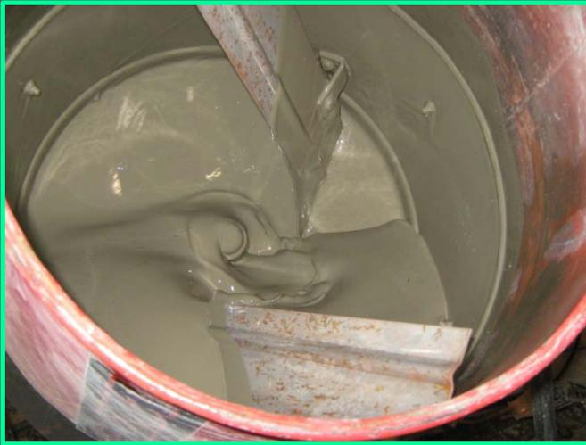
*Slurry in rotary type mixer*
