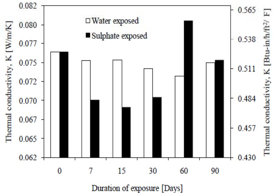
*Thermal conductivity of plain (0.0% fibre) cement-based foams after immersion to sulphate bath and water bath for various duration of exposure (457 kg/m<sup>3</sup>).*
