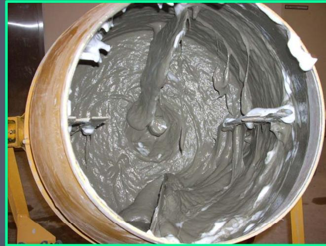
*Mixing foam with slurry*
