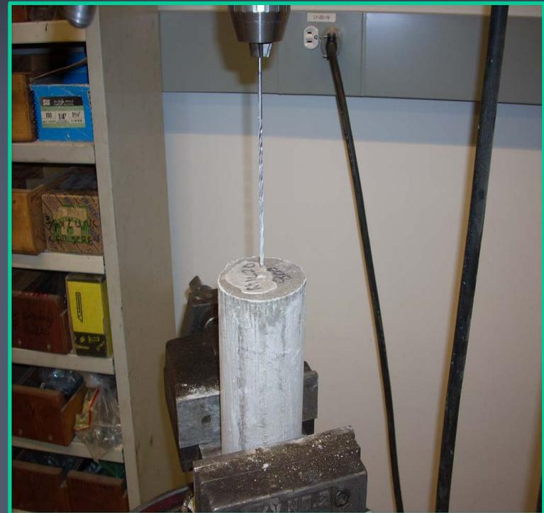
*Drilling the sample to accommodate the thermal probe*
