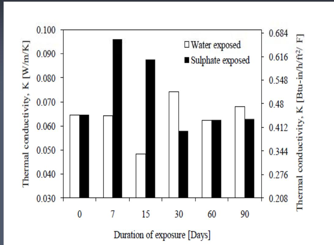
*Thermal conductivity of fibre reinforced (0.2%) cement-based foams after immersion to sulphate bath and water bath for various durations of exposure. (cast density =  $475 \text{ kg/m}^3$ ).*
