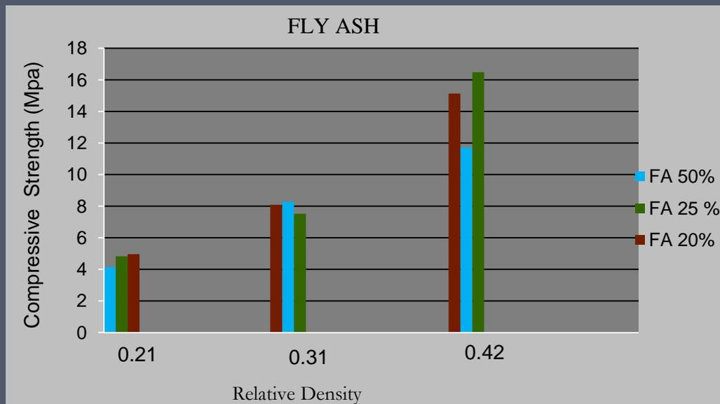
➤ Increased amount of Fly Ash reduces the compressive strength.
