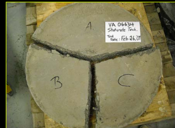
Panel broken into three pieces with typical Y yield line failure pattern
